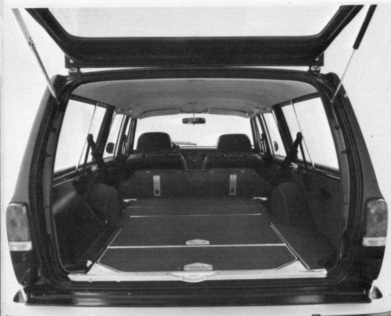
145 rear compartment holds up to 70 cubic feet of cargo with a twin-lid underfloor compartment. Fully carpeted flat floor has a maximum length of 74 inches. The rear door opens upward, assisted by a gas-filled cylinder. The left side brace is equipped with a safety latch.
