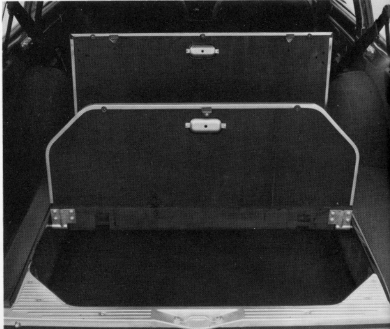
145 rear compartment holds up to 70 cubic feet of cargo with a twin-lid underfloor compartment. Fully carpeted flat floor has a maximum length of 74 inches. The rear door opens upward, assisted by a gas-filled cylinder. The left side brace is equipped with a safety latch.
