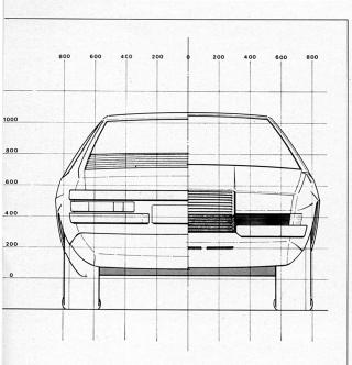
This unique prototype presented by Carrozzeria Coggiola at the 1971 Paris Auto Show is based on the 1800 ES Volvo coupe chassis, whose body recently underwent an important re-design. The production underbody was not modified, but appropriate solutions allowed a better exploitation of its dimensions and structural features, to the ends of a substantial increase in interior roominess. Interior completely lined with leather, air conditioned.
