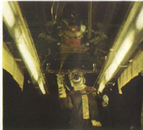
The 1800 S is treated with underbody sealing before it leaves the factory.
