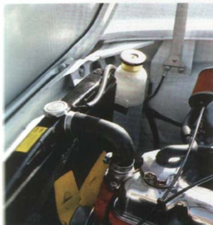
Sealed cooling system. Resistance to temperatures down to -40^{\circ}\text{C} ( -40^{\circ}\text{F} ).
