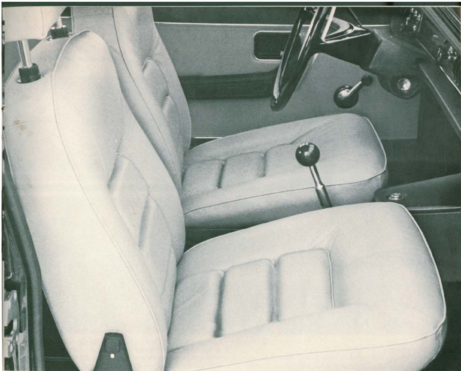
Leather upholstered 164 seats can, in addition to back and forth adjustments, be raised or lowered.
