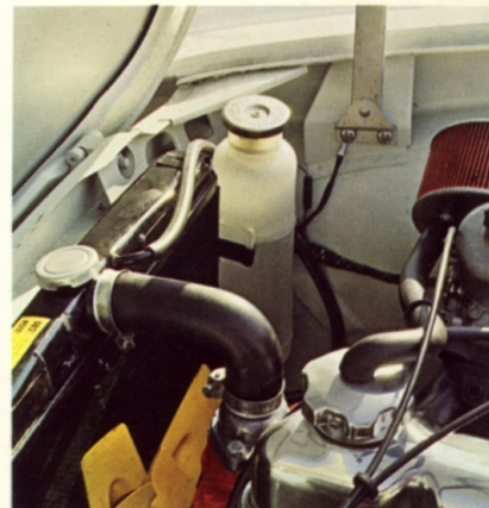
The sealed cooling system keeps the radiator from blowing its stack.
