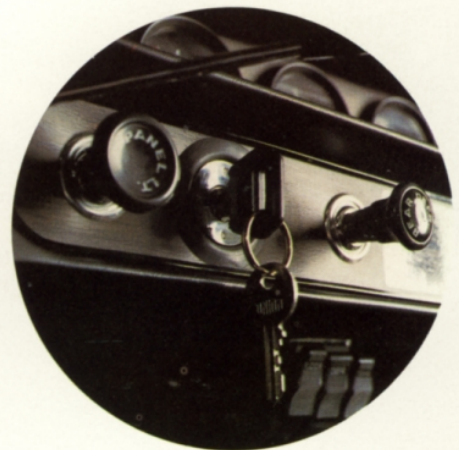
A warning buzzer will remind you if the ignition key was left behind.
