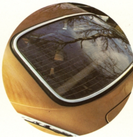
Electric rear window defrosting dries up mist and melts ice. With 150 watts of power.
