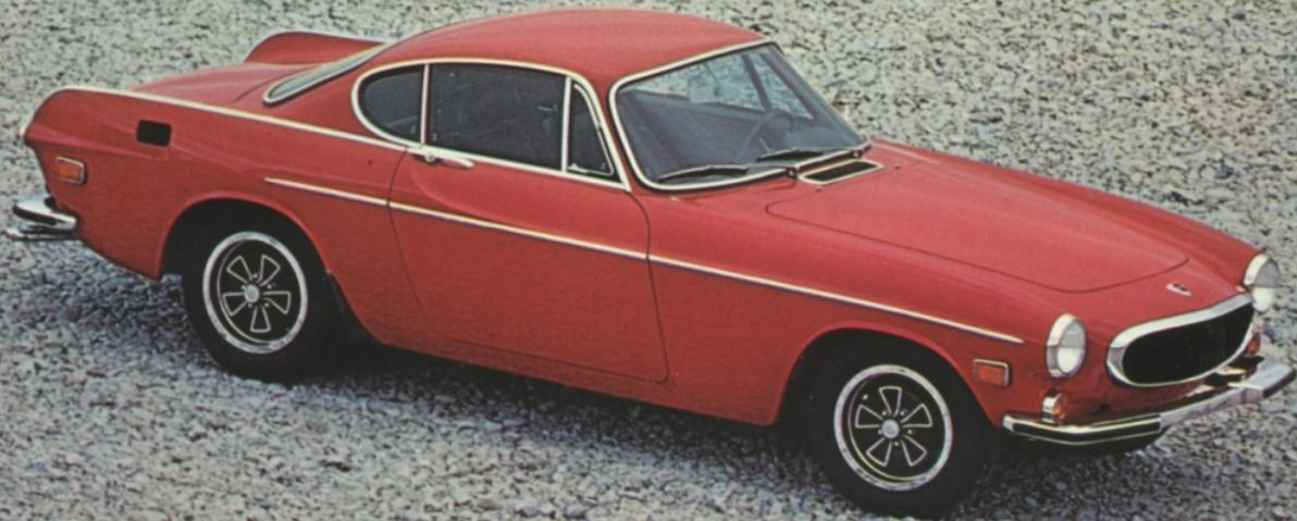
The little computer is what makes the Volvo 1800E run so efficiently. It exactly proportions the gas and air mixture for better performance and economy. Now you can match the B20E engine to an automatic transmission.
