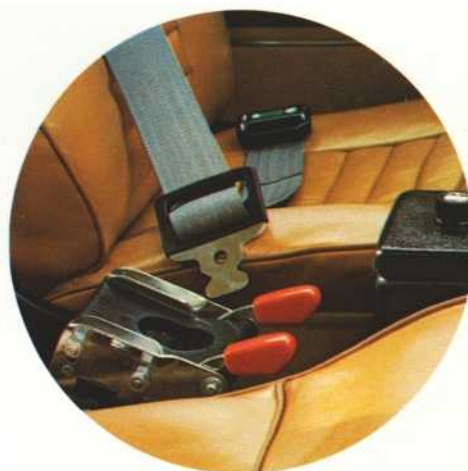
The front seats have factory-fitted three-point safety belts. Convenient snap-action locks.
