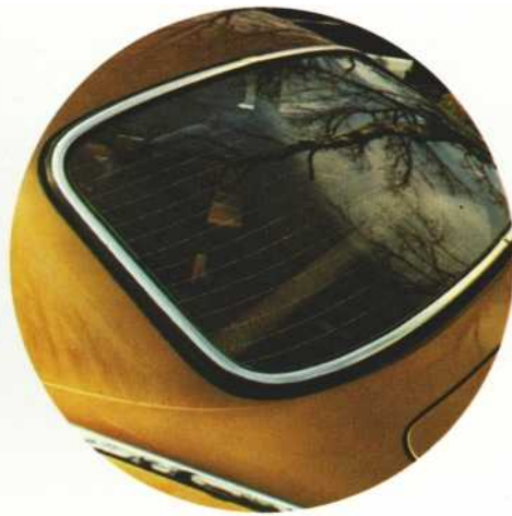
The rear window is electrically heated. So you can always see the cars you've just passed. Through mist and frost free glass.
