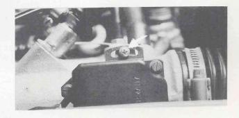
Adjusting throttle valve switch:
