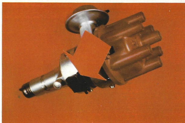
Fig. 17. Distributor (arrow indicates position of trigger contacts).
