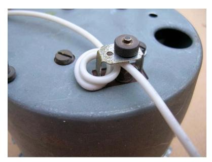
If you are using the actual ignition signal to calibrate the tach you can just wind a couple turns of the ignition wire through the clip. You do not need to use the plastic piece that is installed in the white wire. For some tachs I have seen a need to wind an extra turn, one more than the 1-1/2 turns originally used, in order to get the tach to respond. It's easy to do if you don't use the plastic piece.
