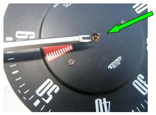
When replacing the needle just press it on to the pivot pin. Initially install it slightly above the "0" position and don't press it on very hard. Then rotate it into final position at "0" and then press it a bit more firmly on with just finger pressure .
