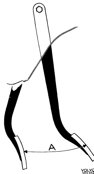
Fig. 5-62. Pedal travel A=approx. 152 mm (6")
