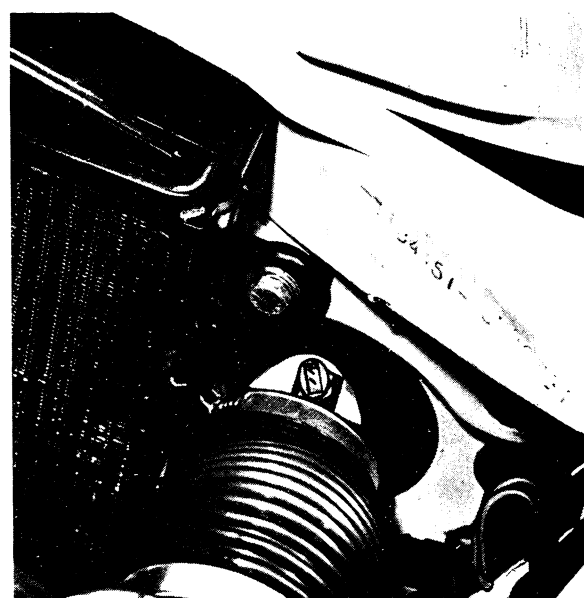
Fig. 2-75. Intake air temperature sensor (connection removed)
