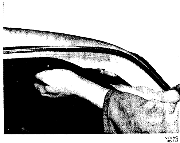
Fig. 8-42. Fitting sealing strip for door opening
