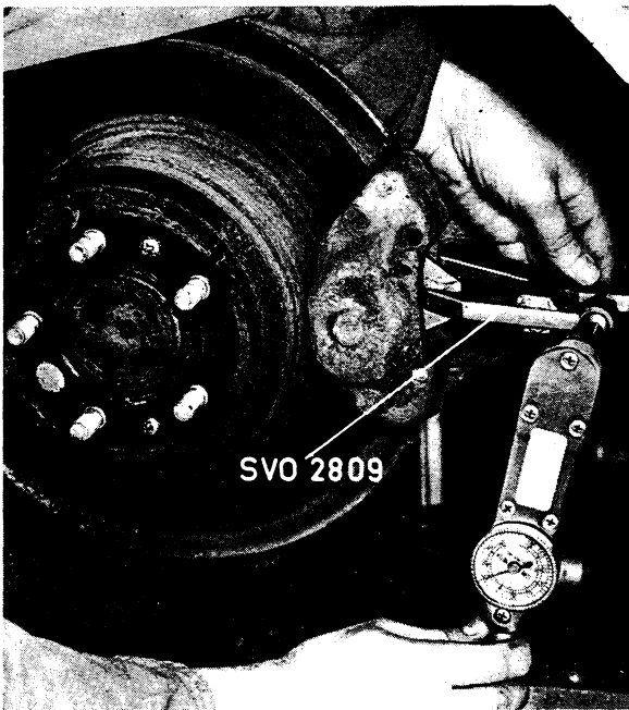
Fig. 5-17. Pushing in piston with A.S.B. device
