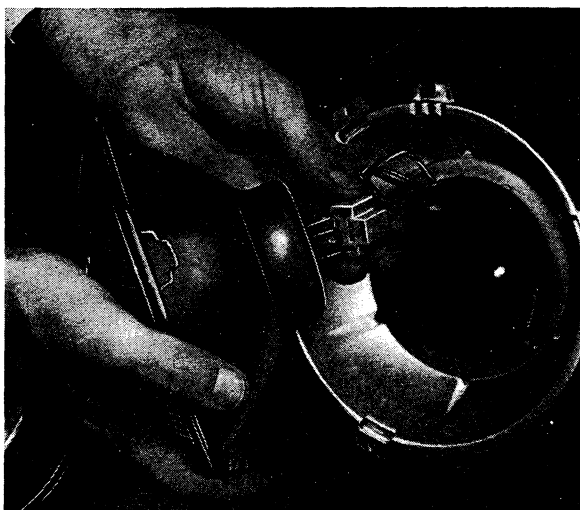
Fig. 3-82. Removing connection contact
