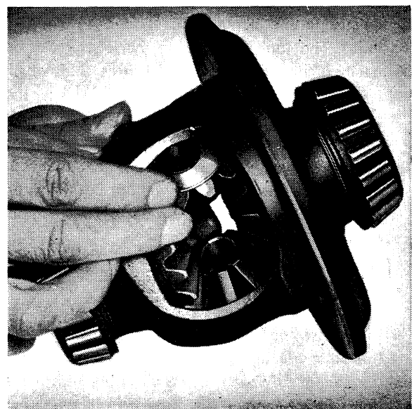
Fig. 4-144. Fitting differential gear
