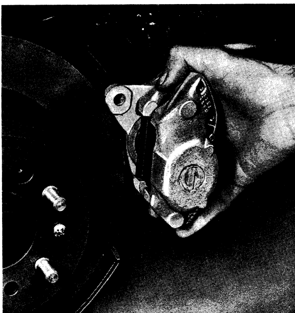
Fig. 5-26. Removing rear wheel brake caliper
