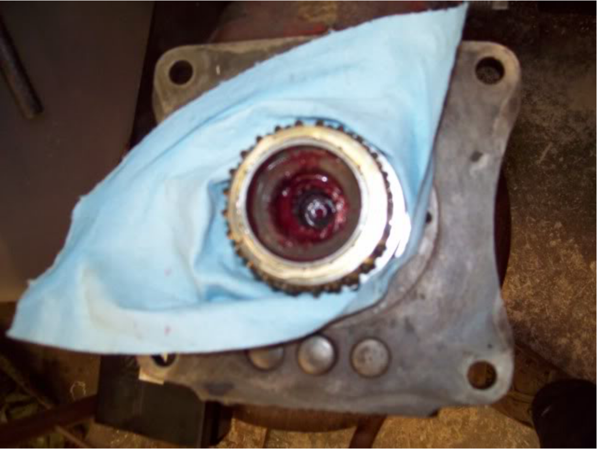
With this shaft rebuilt, and the bearings & grease routine repeated and the input shaft installed, we are ready to insert the output shaft. Careful, now. I realized the big synchro was on backwards later making the shift lever forks misaligned.
