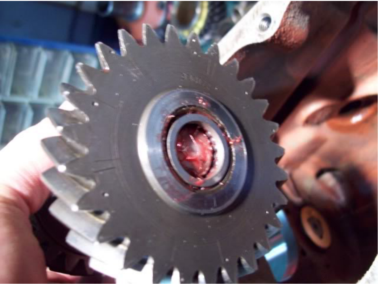
The layshaft washers are shellaced with some oldschool gasket shellac and tacked in position in the 'box. The rod can be used for accuracy.
