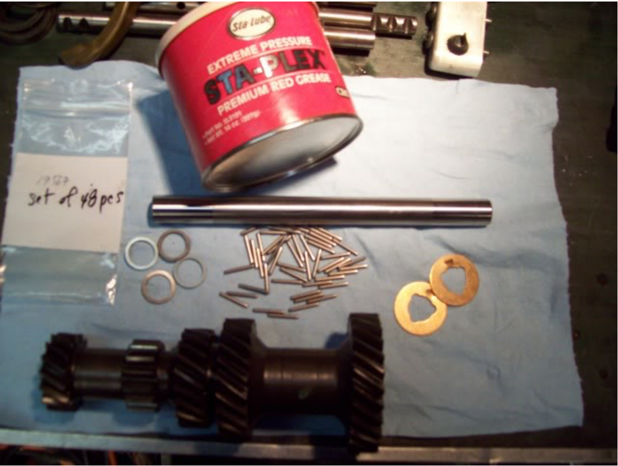
First we make a shaft slightly smaller than the original in diameter.
