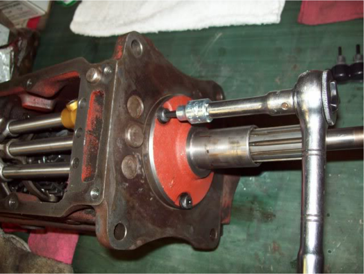
Removal of the speedometer drive gear assembly retainer bolt, the gear assembly, then the rest of the output bearing cover bolts:
