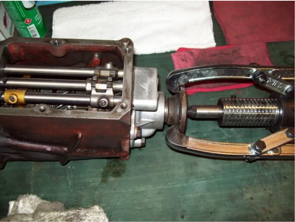
Removal of the bearing cover, input shaft side:
