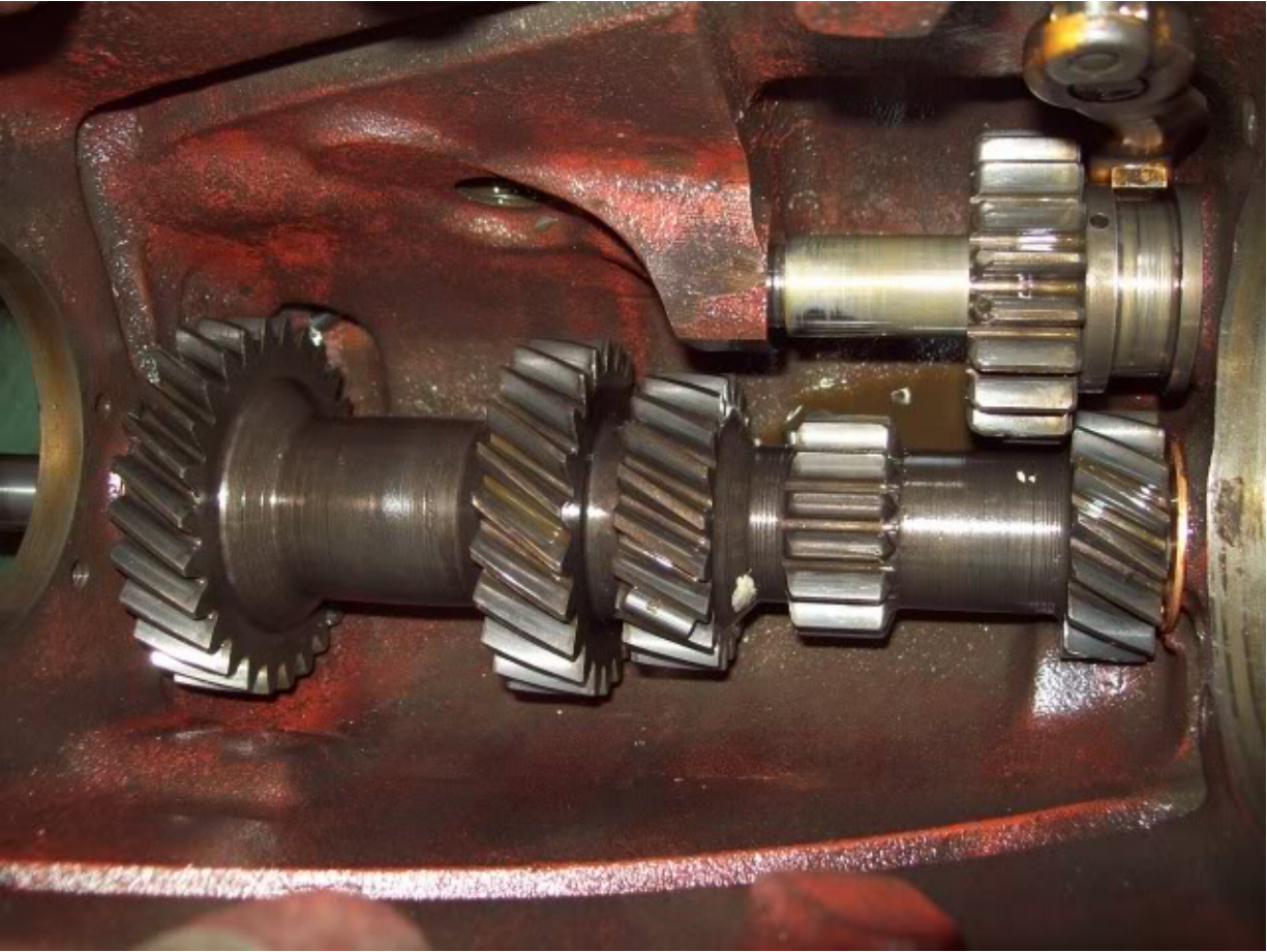
Oh wow, I chunked 4 teeth off the countershaft, so that's what this feels and sounds like:
