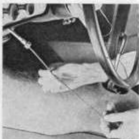
Fig. 19. Lubricating the speedometer cable.
