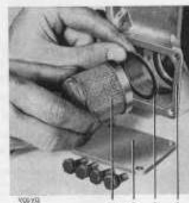
Fig. 14. Removing the overdrive oil strainer.
