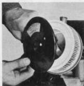
Fig. 12. Replacing the air cleaner element (right-hand drive).
