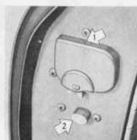
Fig. 23. Door lock. 1. Lubricating hole for lock (silicon oil) 2. Door latch (paraffin wax)
