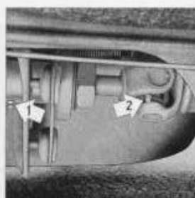
Fig. 27. Centre universal joint. 1. Splined shaft 2. Universal joint
