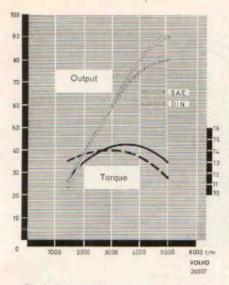
Fig. 4. Output and torque curves for B 18 D r/m = r.p.m.
