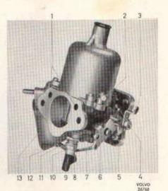
Fig. 10. Carburettor viewed from right.
