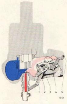
Fig. 15. Carburettor, fast idling.
