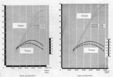
Fig. 3. Output and torque curves for B 18 B. r/m = r.p.m.
