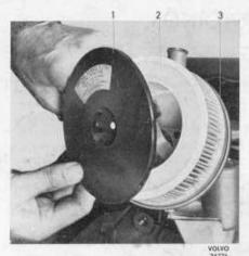
Fig. 27. Replacing air cleaner element (P 120 right-hand drive)
