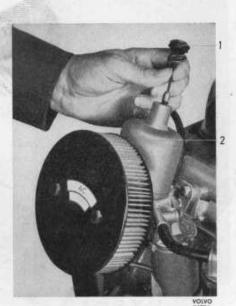
Fig. 18. Checking the oil level.
