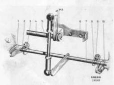
Fig. 25. Intermediate shaft and levers.
