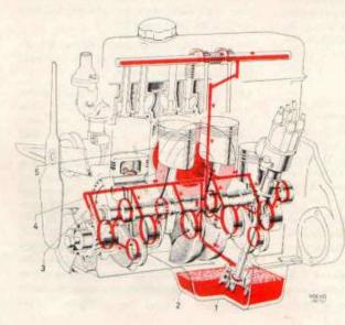
Fig. 5. Lubricating system.
