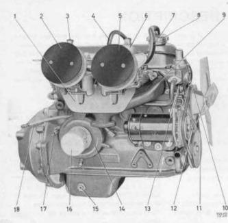
Fig. 2. The engine viewed from the right. (Oil cooler only on B 18 B.)
