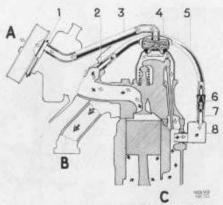
Fig. 7. Positive crankcase ventilation (B 18 B).
