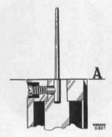
Fig. 19. Attachment of fuel needle.
