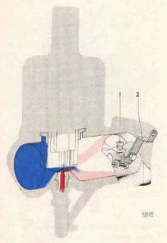
Fig. 14. Carburettor, idling
